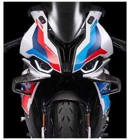
maximum speed that is as high as possible and absolutely necessary for winning races, there was another objective in the technical specifications of the M RR: to establish the best possible contact of the wheels with the road - especially when accelerating. The M winglets on the trim front, which were developed during intensive testing on the race track and in the BMW Group's wind tunnel
