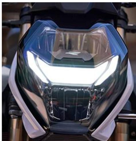
The adaptive turning light, which is unique in the mid-range, works by switching on additional LED elements in the main headlight that are fitted with their own reflectors, depending on the banking angle. It is activated from an inclined position of more than 7° and a speed of more than 10 km/h. The additional lighting effect can be perfectly experienced up to a banking angle of 25°.
