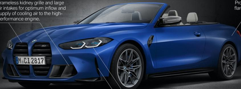
Frameless kidney grille and large air intakes for optimum inflow and supply of cooling air to the high-performance engine.
