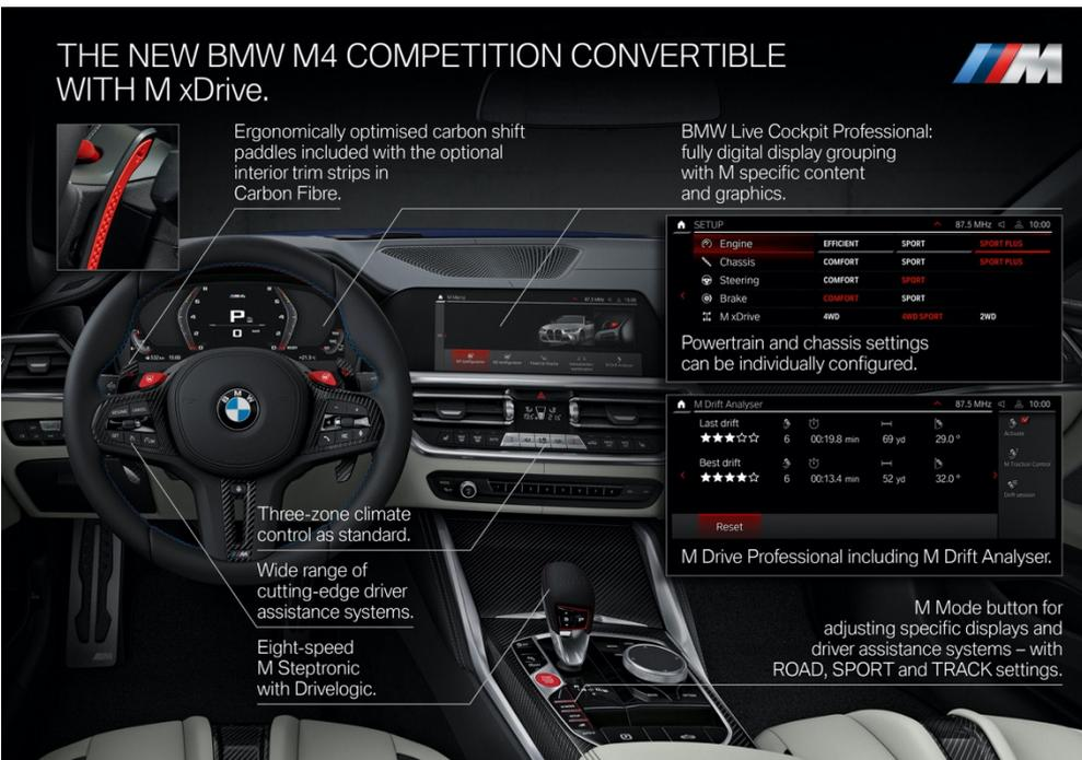
**Ergonomically optimised carbon shift paddles included with the optional interior trim strips in Carbon Fibre.**
