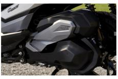
The entire drive unit of the new BMW mid-size scooter has been completely newly developed and includes a directly integrated CVT gearbox as well as a secondary drive in the form of a drivetrain swing arm. The liquid-cooled single-cylinder engine has a capacity of 350 cc, derived from an 80 mm bore and a 69.6 mm stroke. Its rated power output is 25 kW (34 hp) at 7 500 rpm and the maximum torque of 35 Nm is reached at 6 000 rpm. The maximum engine speed is 8 800 rpm.
