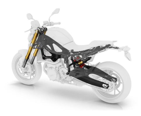
"By adjusting the steering head angle, offset and castor, we were able to achieve a particularly sporty suspension design for the road models. Optimum design of the respective ergonomic triangles allows pronounced segment-specific differentiation while at the same time offering great possibilities in terms of individualisation".
