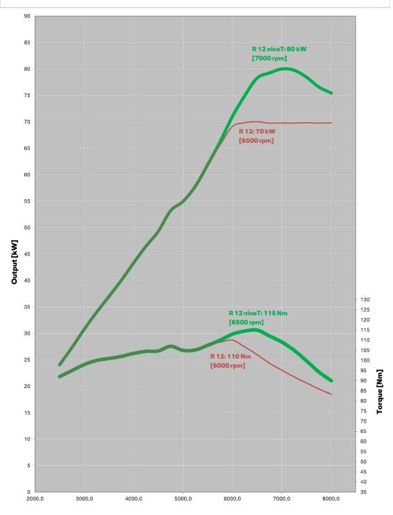
Engine speed [rpm]
