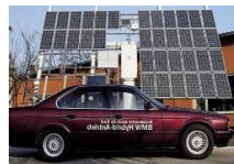
1994: BMW 518i Parallel-Hybrid with NiMH Battery
