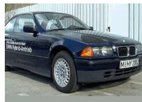
1995: BMW 316i Serial Hybrid with NaNiCl Battery
