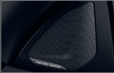
The harman/kardon loudspeaker has a 464W digital amplifier, nine channels, vehicle-specific equaliser and 16 speakers.
