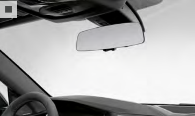
The rear-view mirror features a frameless design and has an automatic anti-dazzle function. This protects the driver from being dazzled by bright lights by darkening its reflective surfaces when light intensity exceeds a defined limit.
