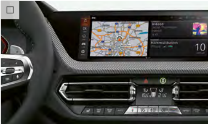
BMW Live Cockpit Professional includes a 10.25" Control Display and a fully digital 10.25" instrument display. Standard for M Sport and M235i xDrive models.
