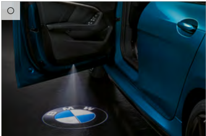
The LED door projectors are activated when the doors are opened. They project an image onto the ground next to the car using an interchangeable slide.
