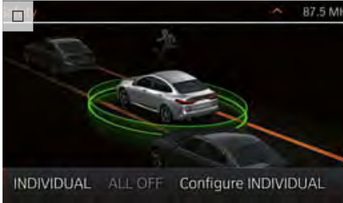
Driving Assistant supports you in numerous driving situations. It includes Lane Departure Warning, Lane Change Warning, Approach Control and Pedestrian Warning with city braking function, Rear Crossing-traffic Warning and Rear Collision Prevention. Only available on models fitted with automatic transmission and Active Cruise Control.
