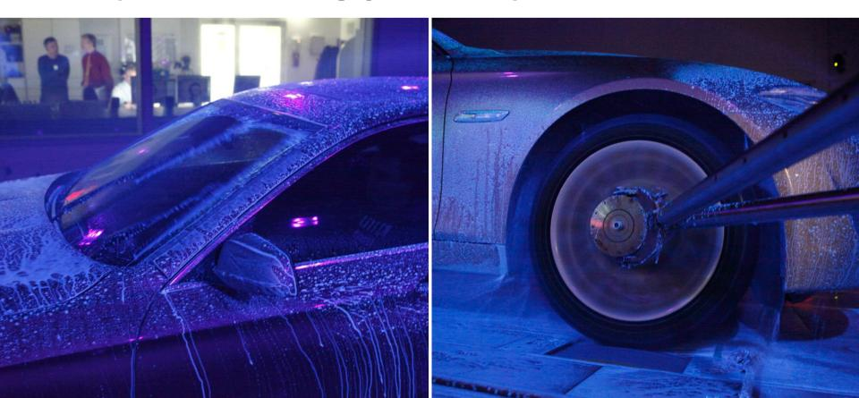
Environmental Wind Tunnel – snow simulation. Snow making (full vehicle) using snow gun.
