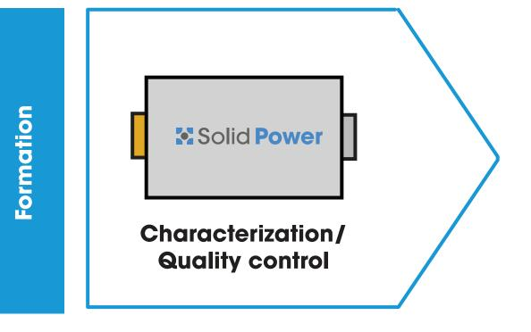
Solid Power's processes eliminate formation cycling and electrolyte filling, which account for 30% and 5% of CapEx in a typical GWh-scale lithium-ion facility
