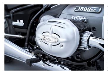
The Option 719 Design Package AERO includes cylinder head covers, front engine cover and left and right intake snorkel covers in aluminum with a brushed, anodized finish. The cylinder head covers feature finely wrought air vents reminiscent of the "streamliners" of the 1920s and 1930s. The highlight is a badge on the front and side covers: This is made of solid copper which is
