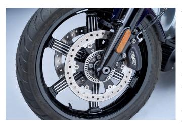
The two Option 719 wheels - AERO and ICON in matt silver and matt black, respectively, provide a refined and sophisticated look to the R 18 and R 18 Classic. The cast alloy wheels feature a six-spoke design. The milled ribs of the spokes are a real eye-catcher. The milled areas give the aluminum a contrast to the painted surfaces - hence the name Contrast Cut.
