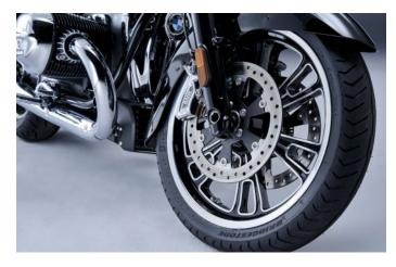
The R 18 B and R 18 Transcontinental feature cast light alloy wheels. The 3.5 x 19-inch front wheel is equipped with a 120/70 R 19 or 120/70 B 19 tire (depending on the manufacturer), while a 180/65 B 16 tire is mounted on the 5.0 x 16-inch rear wheel. Original BMW Motorrad Accessories offers additional rims in chrome, Machined
