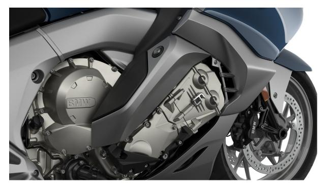
Six-cylinder in-line engine with new engine control, knock sensor system, revised emissions and engine drag torque control.
