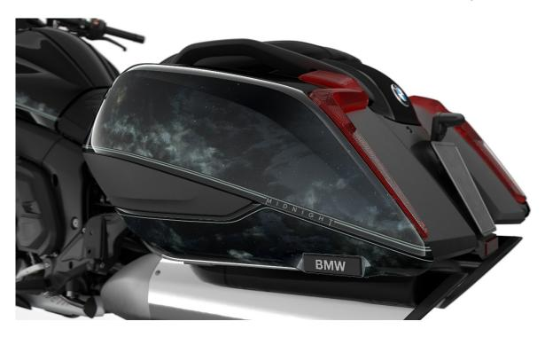
Backing films, which are activated in a water bath, are used as the medium for the later pattern or graphic. The object to be coated is pressed on to the film in the water bath and immersed. During this process, the pattern or graphic on the backing film is
