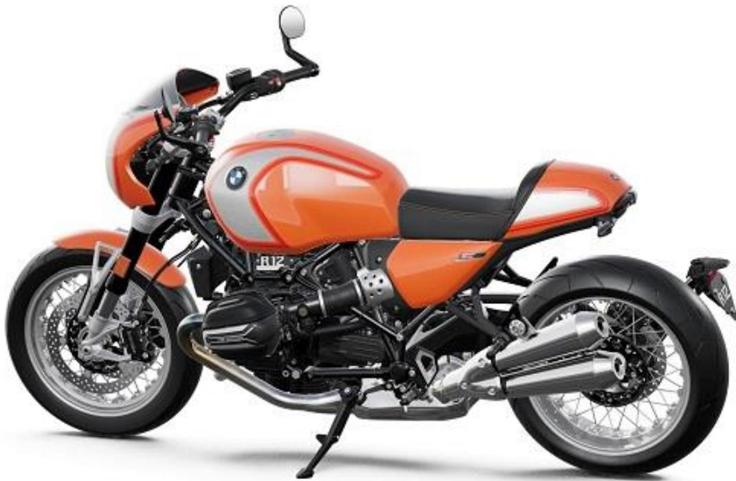
U.S. model with standard short rear tail and swingarm mounted license plate frame.
