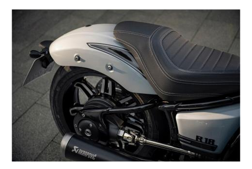
In order to ensure a more comfortable ride, the rear shock has new spring/damping rates. This was tuned to work together with the new 18-inch rear wheel and the new 180/55B18 tire to match. Another new feature is the USB-C charging socket.
