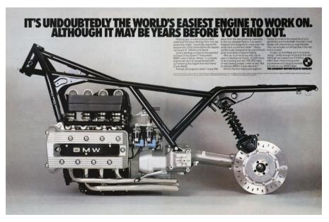
In late 1983, BMW would enter another crucial segment, supplementing its longstanding boxer twin lineup with allnew K bikes powered by water-cooled three- and four-cylinder engines. "Even
