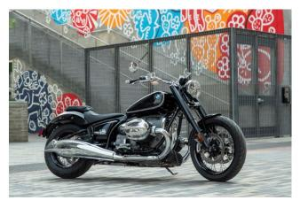
The R 1200 C had no direct successor, but in 2020 BMW reentered the cruiser segment with the retro-style R 18. Like the R 1200 C, it used BMW's largest-displacement air/oil-cooled engine, this time a massive 1,802cc boxer twin. Its distinctive styling—by a team led by Ola Stenegard,
