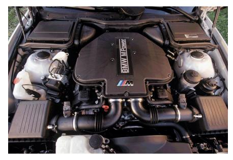
Even more surprisingly, the M5's production-based S62 V8 engine made its way to the racetrack. With the six-cylinder S50 no longer competitive, Tom Milner's engineers adapted the S62 V8 to the Jet Racing
