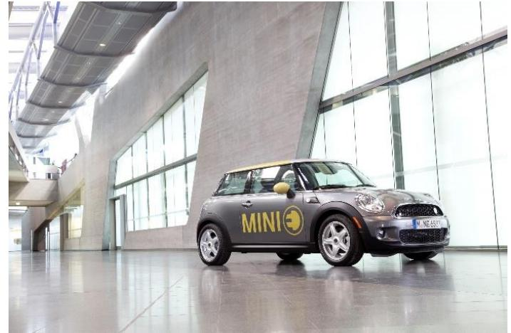
That powertrain used 1,088 lithium-ion cells strung together within a 573-pound battery pack, which gave the MINI E the equivalent of 201 horsepower. It could accelerate from zero to 62 mph in 8.5 seconds en route to a top speed of 95 mph. Needless to say, it would have to be driven far more sedately to achieve its claimed 156-mile range.
