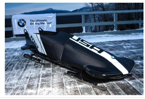
performance, though most improvements would be gained through aerodynamic efficiency. In this area, Scully's team was able to compare data from CFD testing with that generated in the wind tunnel, correlating the two data sets to ensure accuracy and reduce drag from specific components.
